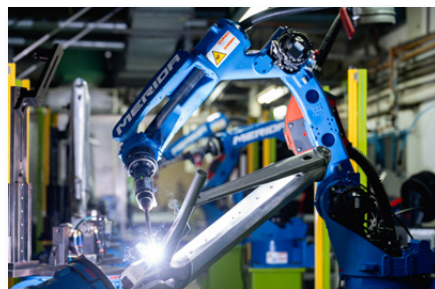
Bicycle welding by robot
