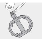
Apply assembly paste to the crank arm threads, and the threads and contact surfaces of the pedal axles.
