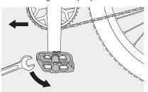
The left pedal has a left-hand thread. Screw in the axle counter-clockwise and then tighten it with a pedal wrench.
