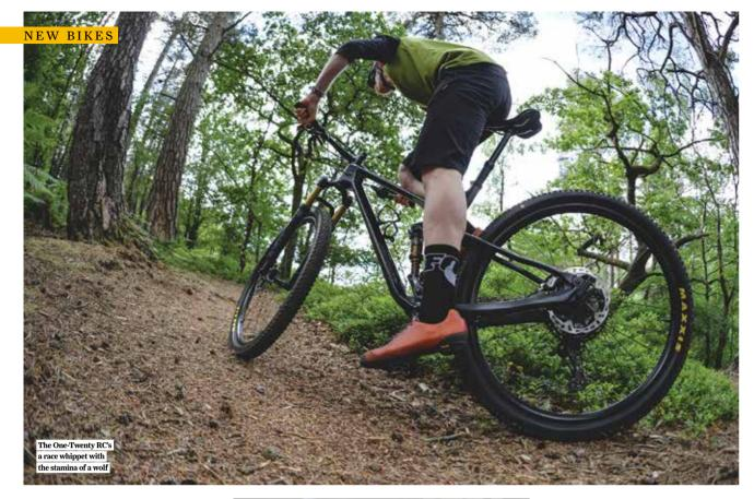
bike costs £3,700 more than the next model down with an alloy rear end. Still, Merida has created a carbon rear end that combines elegant profiles with dimensions that scream stiffness, adding race-level performance while contributing towards the 9.9000's impressive 10.71kg (23.61lb) weight.
