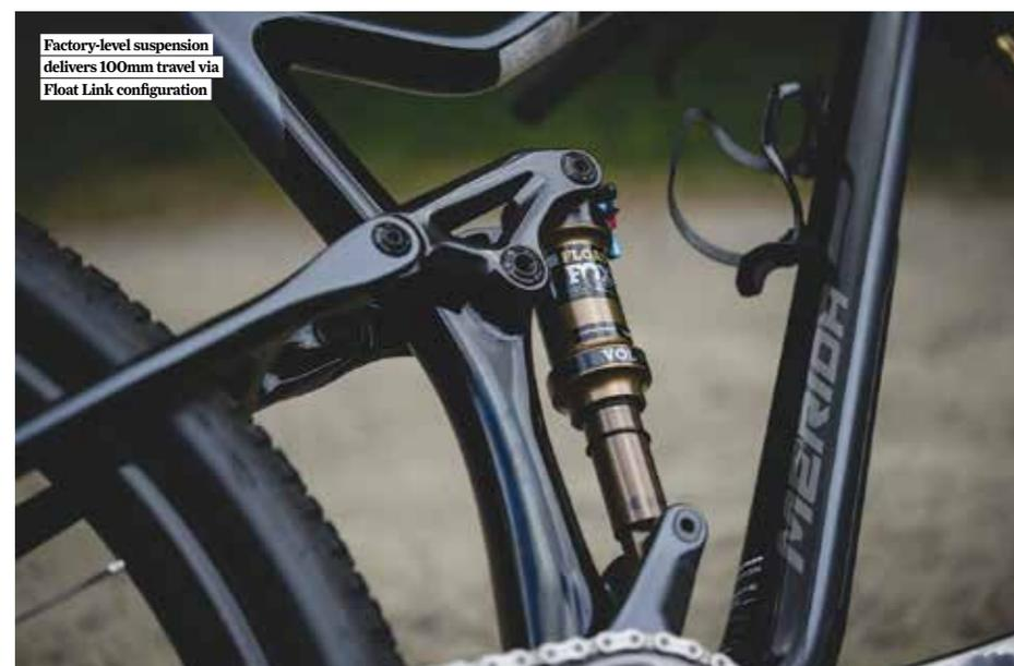
Factory-level suspension delivers 100mm travel via Float Link configuration
