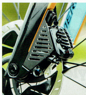
The fork has an integrated disc cooler to improve braking
