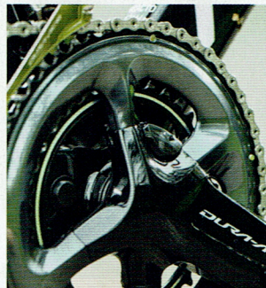
The Reacto comes fitted with a Dura-Ace power meter chainset
