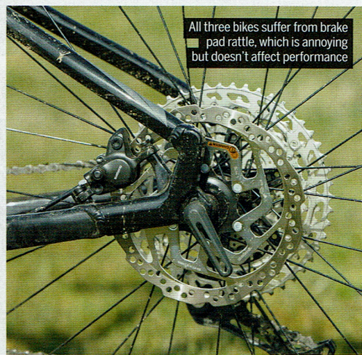
We banged our heels on the chainstays, which sweep out to accommodate the 148mm rear hub
