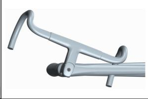
Adjust headeset bearing play by sligthly tighten the headset preload bolt [1]
