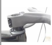
HINT: Do not tighten the expander plug before sliding the shim and stem over the steerer – this will help to get all parts slided in correct position more easily.
