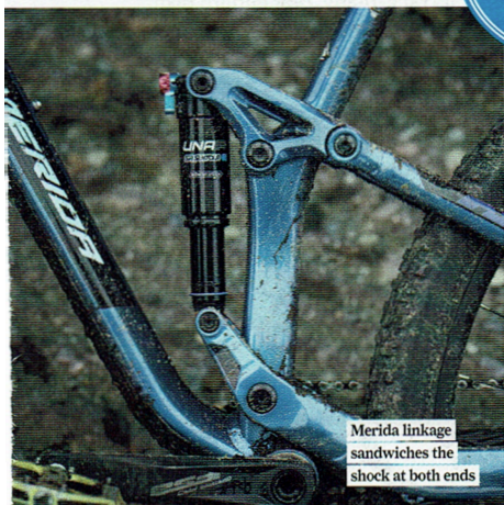
Burly Suntour XCR 34 tracks true but doesn't flinch on small hits
