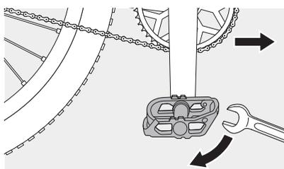
Insert the axle of the right pedal by hand and turn it clockwise slightly. Then tighten it with a pedal wrench or a long 15 mm open-jaw wrench.
