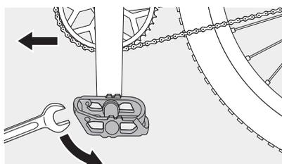
The left pedal has a left-hand thread. Screw in the axle counter-clockwise and then tighten it with a pedal wrench.
