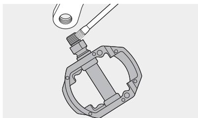
Apply assembly paste to the crank arm threads, and the threads and contact surfaces of the pedal axles.
