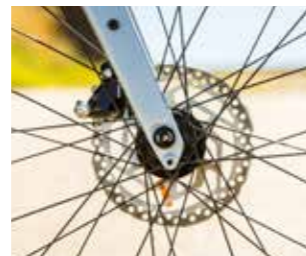
TOP Cables route externally, but there's provision for internal Di2 cables ABOVE I was impressed with the RS405 hydraulic brake performance
