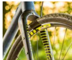
TOP Fixtures and fittings for any configuration you could want ABOVE The Jari fork routes the brake hose internally
