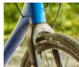
TOP A tall front end with a short steering cockpit works well ABOVE The Merida's full carbon fork is drilled to fit full-length mudguards
