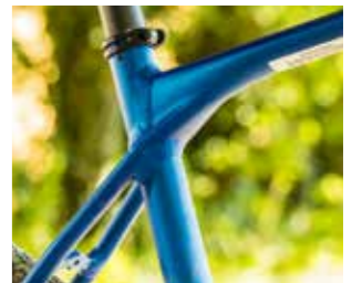
BELOW Hydroformed and shaped alloy give the Silex a touch of class
