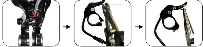
8. Push the lever for 5-10 times to eliminate possible cable loose.
