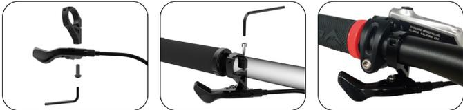
Install lever only at the left handlebar side (rider's left hand). Use 3 mm hex allen key to fix the clamp lever onto handlebar.
