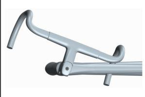
Adjust headeset bearing play by slightly tighten the headset preload bolt [1]
