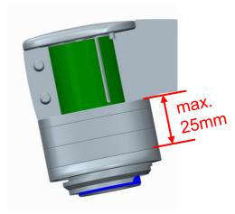
One of the key features of your MERIDA Team SL 1P cockpit is a FORCE DIFFUSER called steerer shim. It increases steerer safety and durability.
