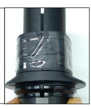
Pre-assemble compression ring [11], neck [9], (if needed spacers [7 & 8]) and shim [10] by sliding the shim from top side through spacers, neck and compression ring.
