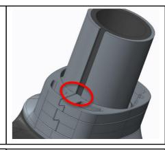
Slide the pre-assembled package of shim, compression ring, neck and possible spacers on the steerer tube.
