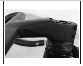
Assemble bearings, compression ring, neck and desired amount of spacers (max. 25mm) like described above.
