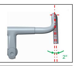
Min Stack height: 7mm between headtube upper edge and stem lower side. Clamping height of stem: 35mm.
