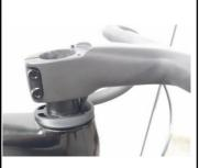
HINT: DΩ not tighten the expander plug before sliding the shim and stem I over the steerer - I all parts slided in position correct more easilu.
