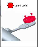
Fix the h-bar adapter [17] with countersunk screw [14]. Tighten with 3Nm
