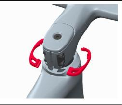
Alternatively, if you don't know exactly your desired heigt of h-bar/stem, you can also keep the steerer longer and assemble spacers above the stem:
