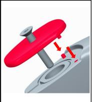
Before tightening the preload bolt, assure the compression ring [11], neck [9], optionally spacers [7, 8] and steerer shim [10] are still correctly positioned. The slice in compression ring needs to point backward and the pin of the neck must engage in this gap. The gap between neck and frame is <1mm.
