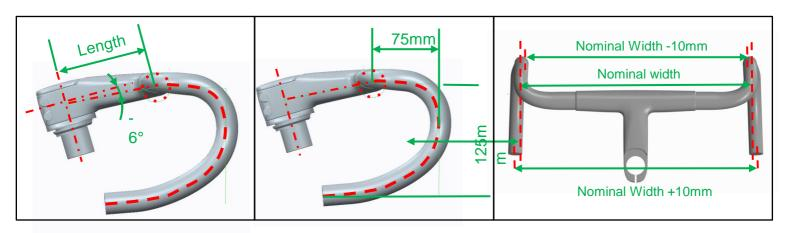
Stem Length: 90, 100, 110, Reach: 75mm Nominal width: 400, 420, 440 mm 120, 130mm Drop: 125mm (measured center to center).
